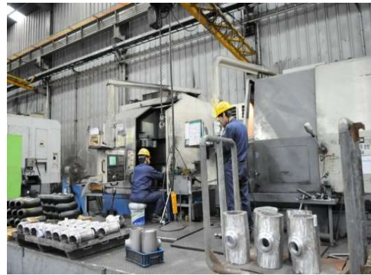
CNC Boring Machine
