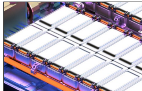
EV Module Housing
