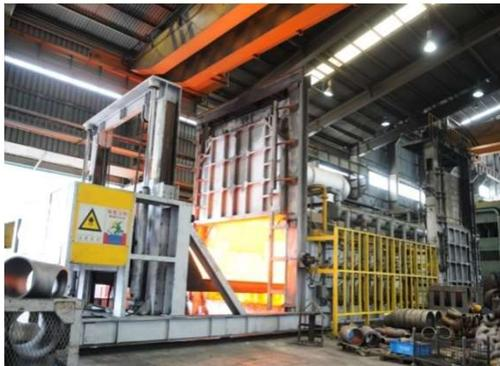
Heat Treatment Furnace For Fitting
