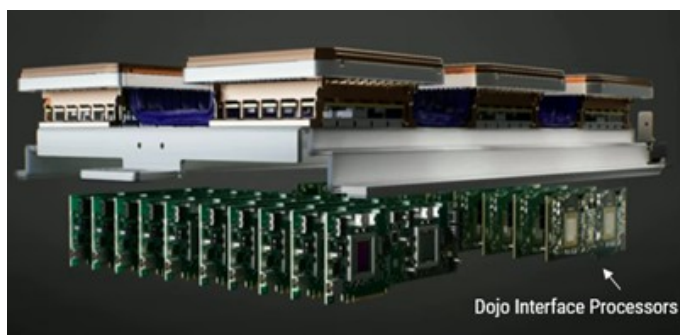
Exhibit 62: 20 Dojo Interface Processors are attached underneath the system tray
