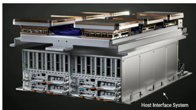
Exhibit 63: The Host Interface connects directly to the Dojo Interface Processors
